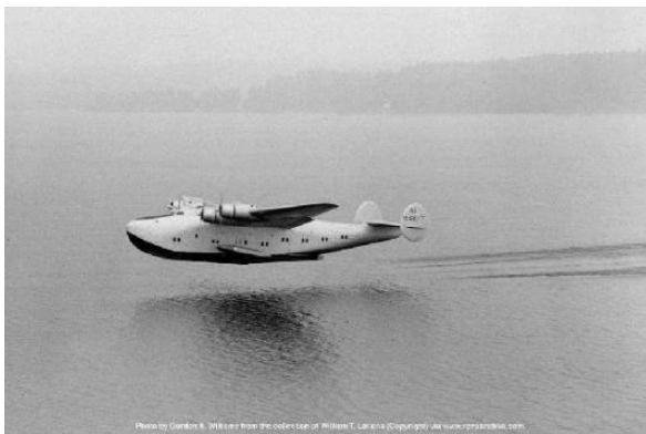
Famed Boeing Test Pilot Eddie Allen conducts a taxi test on Elliott Bay - about 5 Jun 1938. Notice the single (small) vertical fin. The 314 had more than its share of bugs that all needed shaking out before it could enter service.
