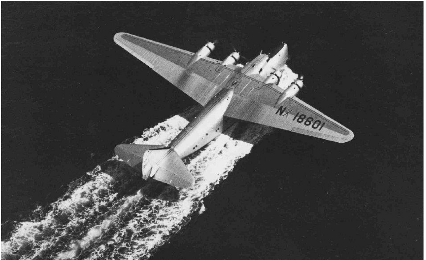
Famed Boeing Test Pilot Eddie Allen conducts a taxi test on Elliott Bay - about 5 Jun 1938. Notice the single (small) vertical fin. The 314 had more than its share of bugs that all needed shaking out before it could enter service.
