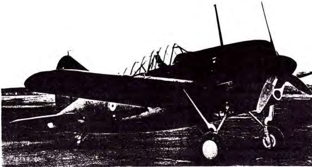
The Belgian Model 339B featured a pointed tailcone which lengthened the Buffalo's fuselage slightly. The carrier style tail wheel and cuffed Curtiss Electric propeller of the F2A-2 have been retained, but the pitot tube has been replaced by an 'L' shaped pitot tube.
