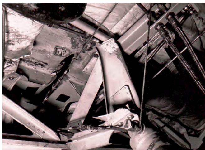
Detached aft cargo door cylinder, blocking the elevator cable.
